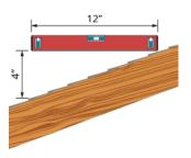
**280.** The slope of the roof shown here is measured with a 12" level and a ruler. What is the slope of this roof?
